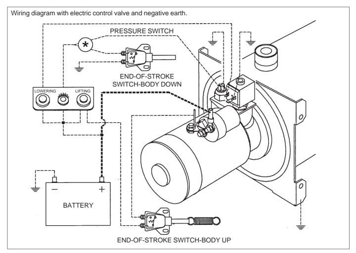
★ The indicator light can be controlled by the pressure switch or by the end-of-stroke switch-body down.
